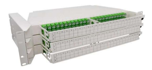
Giganet Rotary Swing out 3U patch panels are designed for the FTTH networks, specifically for the street cabinet where full front access is required. This 3U panel accommodates 144 SC/APC adapters and is loaded with bend insensitive pigtails G657A2 and the complete splicing trays and rooting.
